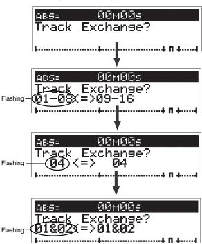
If the **[JOG]** dial is rotated in the condition that "01&02" is displayed, "01&02" ~ "23&24" can be selected. In the same manner, the 2-track unit at right side can be selected by rotating the **[JOG]** dial. For example, if the Track Exchange pattern "07&08<=>01&02" ("01&02<=>07&08") is selected, track 1/2 and track 7/8 will be exchanged upon executing the Track Exchange.
