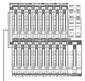
If all the  $1\sim16$  tracks are put in the input monitor mode, the channel 1 ~ 16 [CH STATUS/ CH SEL] keys as well as the [RECORD] key will flash in red.
