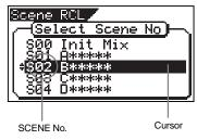
In the above display condition, when executing the DIRECT RECALL or playback by the SCENE SEQUENCE, every time the scene changes, the corresponding scene number will flash.
