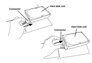
**5** Put back the new hard disk into the VF-16 main unit.
