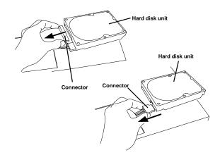
**4** Prepare a new hard disk and Connect the two cable connectors to it with holding the connector section.
