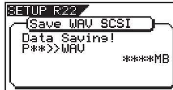
In the case data to be saved cannot be accommodated in a single disc, after the data saving to the 1st disc is completed, it is automatically ejected and "Insert Disk" flashes on the screen, prompting you to remove the 1st disc and to insert the 2nd disc. Inserting the 2nd disc resumes the save operation.
