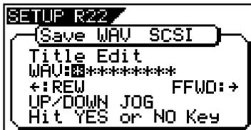
By rotating the [JOG] dial, you can input a desired alphanumeric or symbolic character on a flashing point. To move the flashing point, press the [F FWD] (to the right) or [REWIND] (to the left) key. See the following table for the characters available on VF-16.
