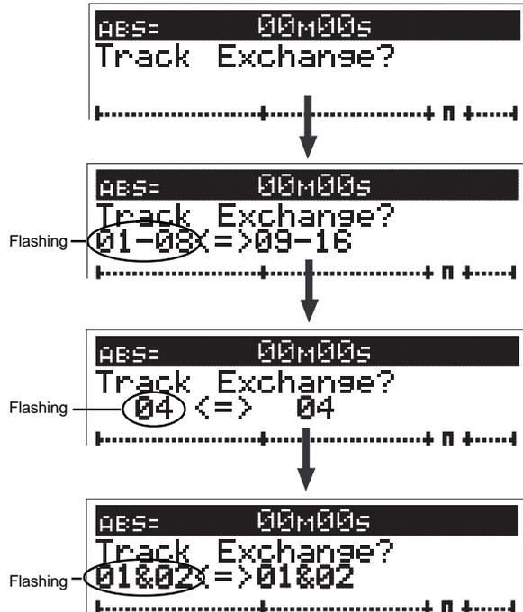
If the [JOG] dial is rotated in the condition that "01&02" is displayed, "01&02" ~ "23&24" can be selected. In the same manner, the 2-track unit at right side can be selected by rotating the [JOG] dial. For example, if the Track Exchange pattern "07&08<=>01&02" ("01&02<=>07&08") is selected, track 1/2 and track 7/8 will be exchanged upon executing the Track Exchange.
