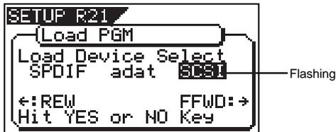
**3 Press the [ENTER/YES] key while "SCSI" is flashing.**
