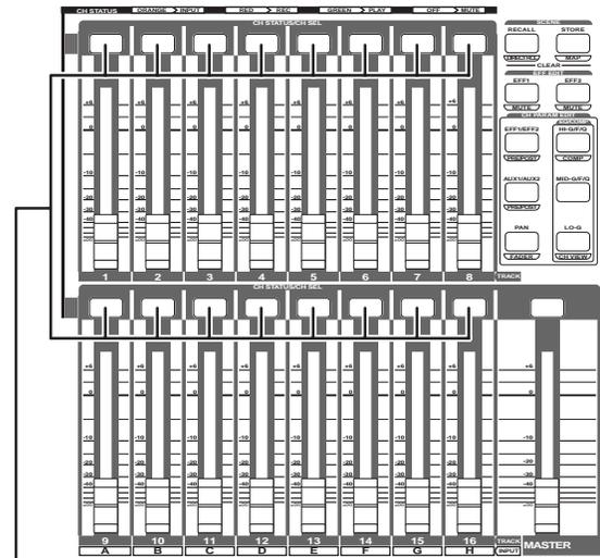
If all the 1 ~ 16 tracks are put in the input monitor mode, the channel 1 ~ 16 [CH STATUS/CH SEL] keys as well as the [RECORD] key will flash in red.
