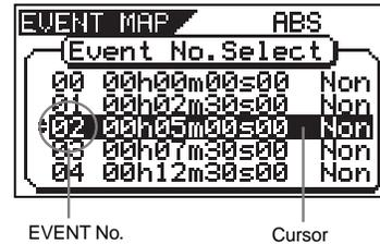
In the above condition, putting the unit in PLAY, F FWD or REWIND mode will flash the Event Number closest to the current location. For example, if the unit is put in PLAY mode in the above display condition, the Event Number 02, 03 and 04 will flash in order.
