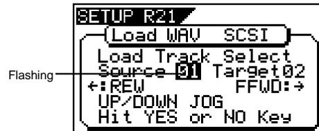
**6 After selecting the track (s) to be loaded, press the [ENTER/YES] key.**
