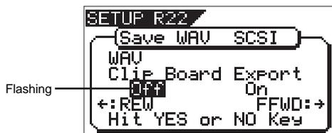
If you would like to save all data from ABS0 to REC END, leave the Clipboard Export function setting to "Off" and go on to the next step.
