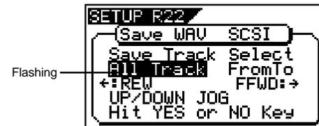
In the above display condition, by rotating the [JOG] dial (or press the [F FWD] key), you can select "From \*\* To \*\*" (where the left field initially flashes) instead of "All Track".
