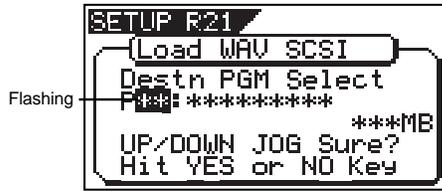
When the screen shows “Title” and “Capacity (MB)”, it indicates that the WAV files to be loaded will overwrite the selected existing program on the VF-16 HD. When the screen shows “Title” and “New PGM”, it indicates that the WAV files will be loaded into a newly created program on the VF-16 HD.
