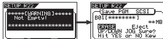
To erase the existing data on a CD-RW disc, select "ERASE" and press the [ENTER/YES] key. If you do not want to erase the data, select "Eject" and press the [ENTER/YES] key. After the disc is ejected, place a blank disc. Rotating the [JOG] dial (or pressing the [F FWD] / [REWIND] key) allows to select either "ERASE" or "Eject".
