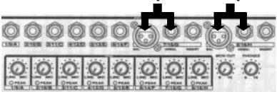
The audio levels for these XLR inputs are controlled using **FADER#15** & **FADER#16** (bottom row)
